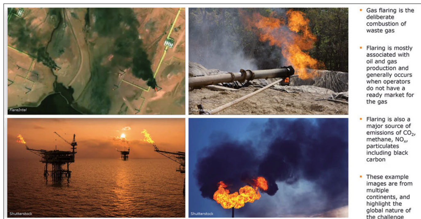
Figure 1: Examples of gas flares from Europe, Africa and the Middle East. Over 10,000 gas flares globally emit more than 1.2 billion CO 2 -equivalent tonnes of greenhouse gases.
