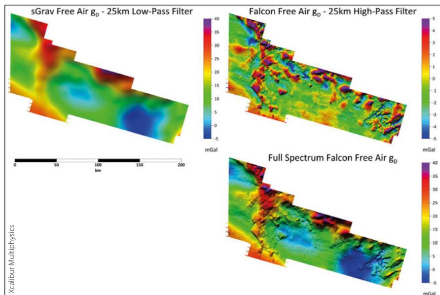
**Figure 4:** The Full Spectrum Falcon solution combines the medium to long wavelength data from the sGrav system (upper left) and the short to medium wavelength data from the Falcon AGG system (upper right). These data are added together to give the Full Spectrum Falcon product (lower right).
