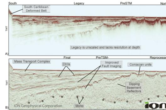
Figure 3: a) Legacy dip-line from offshore Colombia at the SCDB and down-going CLIP. b) The reprocessed data reveals many details within the data, including crustal features and high-frequency stratigraphic units.
