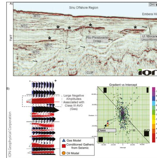
Figure 5: a) A Sinu Offshore example area that features multiple mass transport complexes (MTCs) and seismically bright DHIs in the stratigraphy. A prominent Late Miocene unconformity is present across the region. b) AVO analysis indicates a strong oil/gas signature of a Class III AVO.
