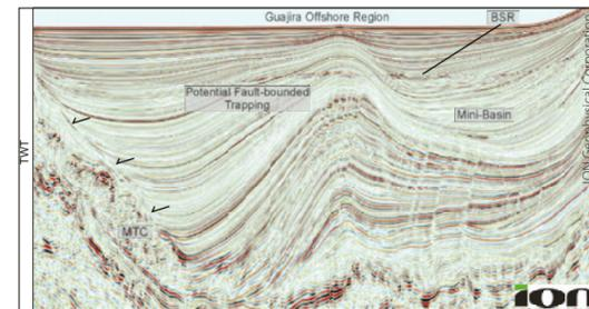
Figure 4: Example line from the SCDB. These units show normal faulting at the anticlinal crest, a bottom-simulating reflector (BSR) and potential trapping mechanisms.
