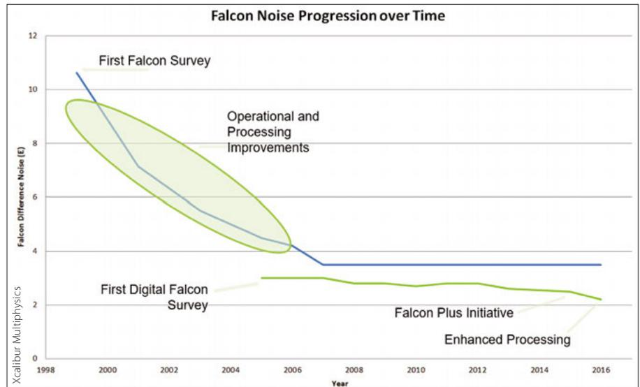
Figure 2: Improvement of noise levels with time obtained with equipment development and enhanced processing techniques.
