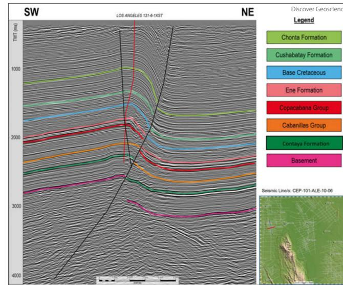
Figure 3: West–east section across the Los Angeles Field structure showing the deep structure and the untested sub-thrust play.
