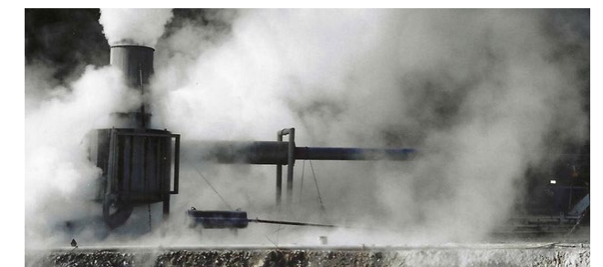
Well testing – an essential element in quantifying the geothermal resource, or reserve. Test conducted at the Patuha geothermal site in Indonesia in 1997.
