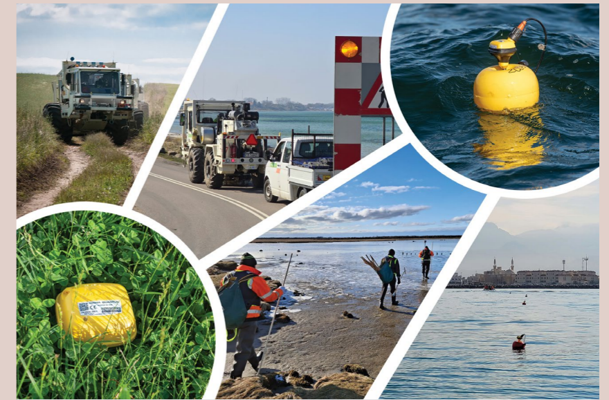
Figure 2: Seismic transition zone surveying includes vibrator operations, onshore data recording by nodes, and offshore data recording by nodes mounted on buoys and surveyors working along the beach.
