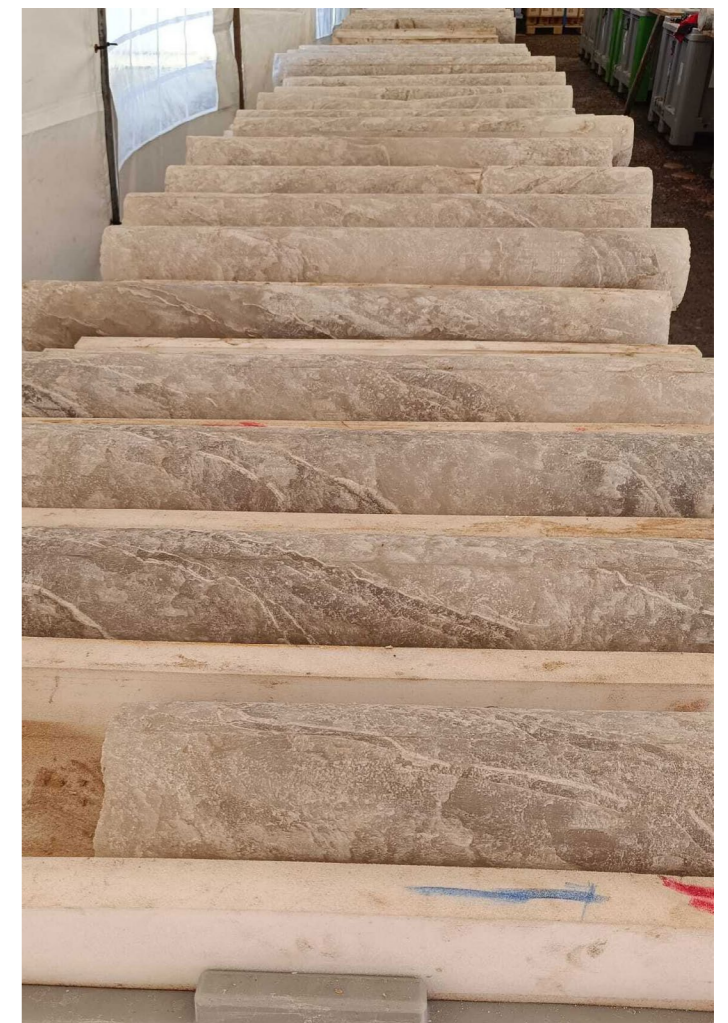
Halite cores from one of the exploration wells drilled to evaluate the Zuidwending salt dome for hydrogen storage readiness.
