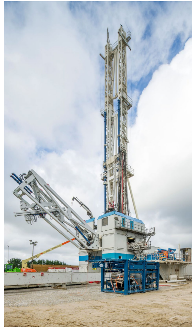
The HAS Innovarig drilled the two wells for the United Downs geothermal project.
