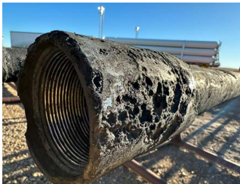
Severely corroded tubing from the 2019 Knappen well.
