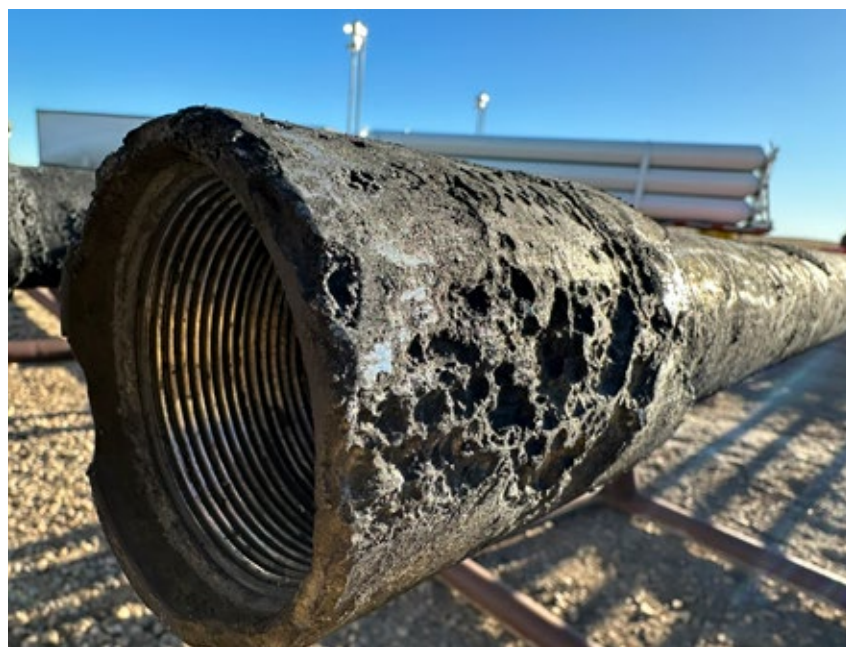
Severely corroded tubing from the 2019 Knappen well.
