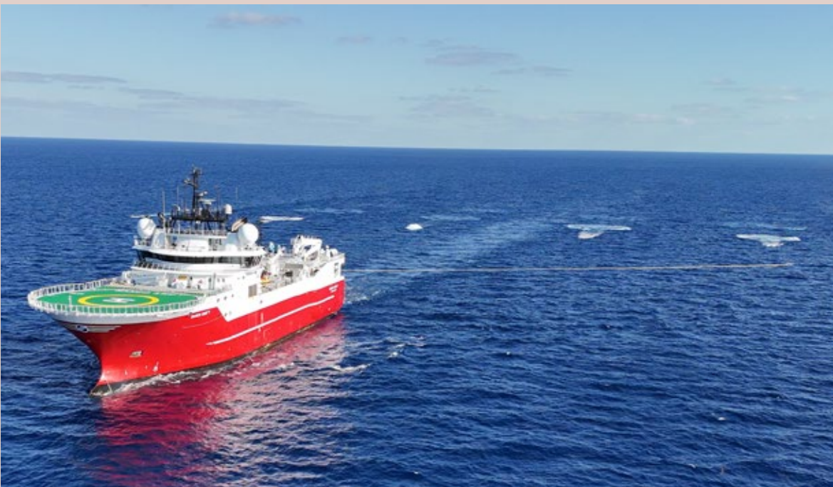
Figure 3: Single source vessel towing 4 Gemini sources, one per gun string during Amendment 4 OBN acquisition.
