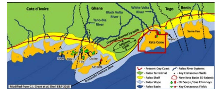
Figure 2b: Map showing the paleo-drainage patterns of the Volta and Tano Basins after the uplift of the Saltpond High in the Campanian. Note how the Volta River systems are now feeding the offshore Tano Basin.
