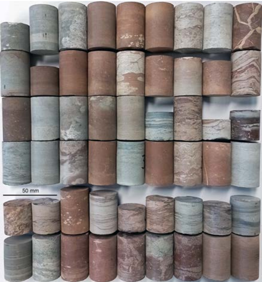
54 plugs from the Haisborough Group of core SM14, prior to porosity-permeability testing.
