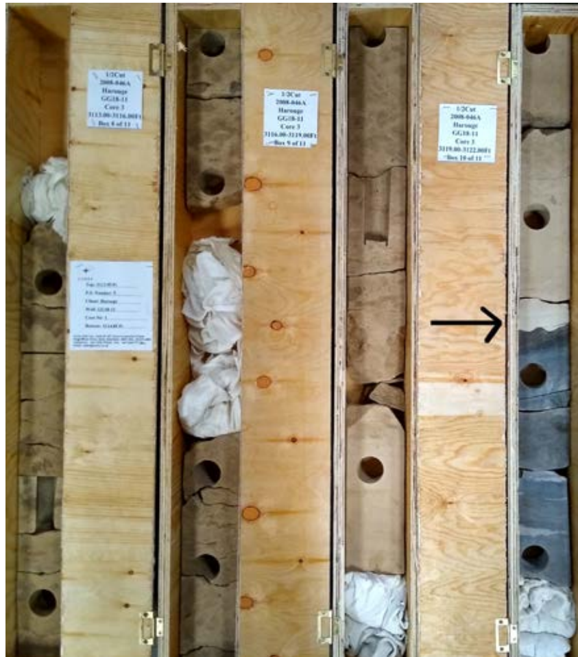
Core 3, GG18-11, 3, 113-3, 122 ft, showing an undulating base of a shallow water carbonate succession overlying anhydrites.
