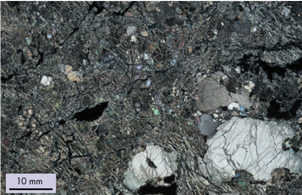
Thin section of serpentinised peridotite under cross-polarised light.
