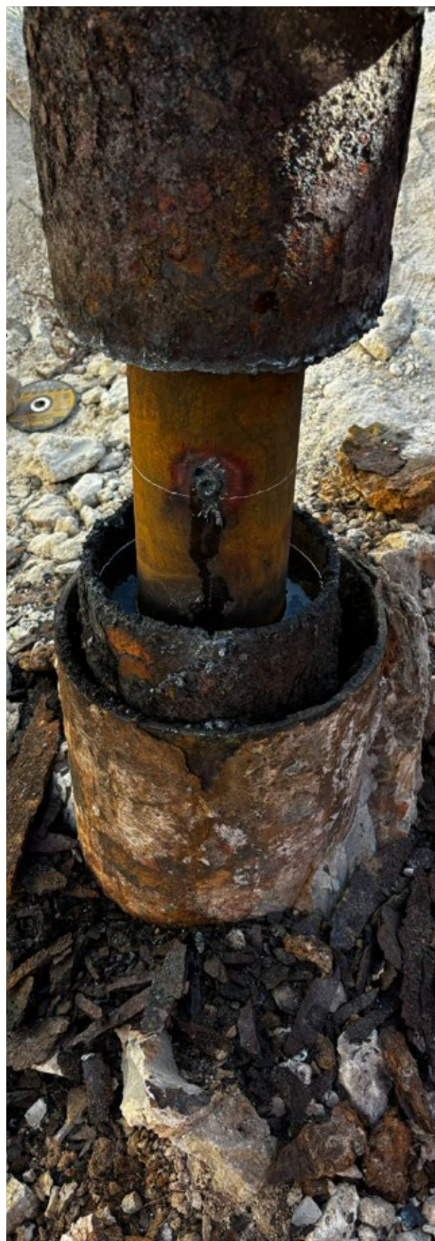
An old Gulf well. Water, oil, and gas were found in all annular spaces at surface.
