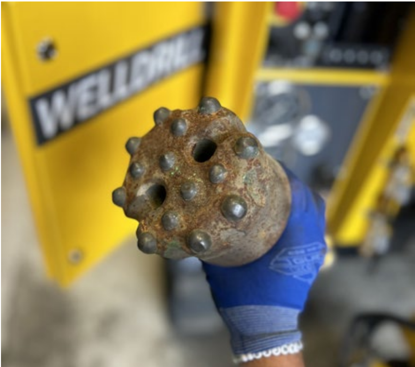
The most used type of bit for drilling shallow geothermal boreholes in Sweden: the hammer bit.
