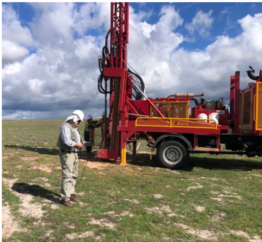
Drilling for soil gas monitoring and soil sampling in Western Australia, August 2023.
