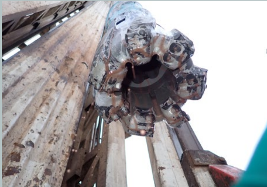
One of Reservoir Group's coring bits showing an irregular placement of the blades to prevent whirling.
