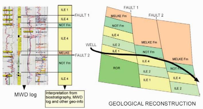
Well trajectory illustrating the need for steering the drill bit because of faults.
