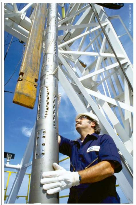
Engineers from Baker Hughes INTEQ on the rig floor following the MWD/LWD tools being run down the well.
