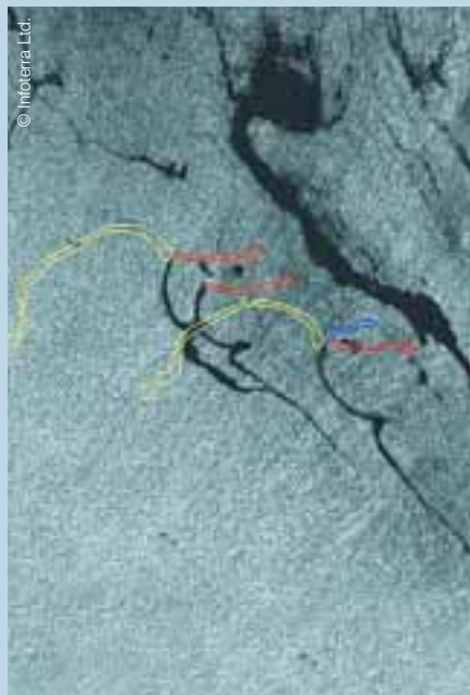
Example of remote sensing used to identify oil seepage in the Caspian Sea. Interpretations from earlier scenes (in colour) show how the seeps have moved over time.
