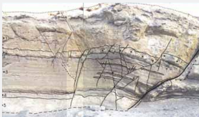
The conventional method of describing faults as simple planes, or curves in cross-section, is evidently misleading.
