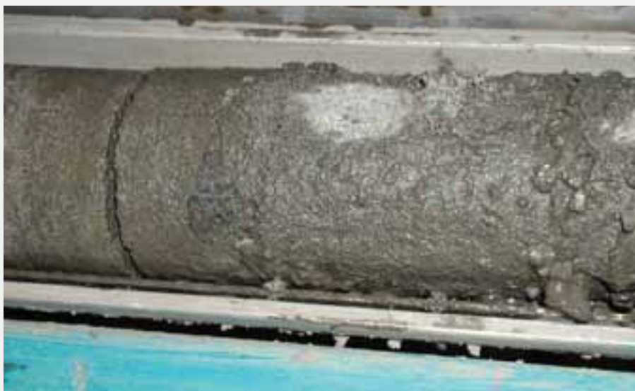
Core from Mallik 1 with bubbling gas hydrates that dissolve as the pressure is relieved.
