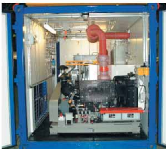
Typical 125 scfm – 350 Barg Diesel Package for Seismic Applications
