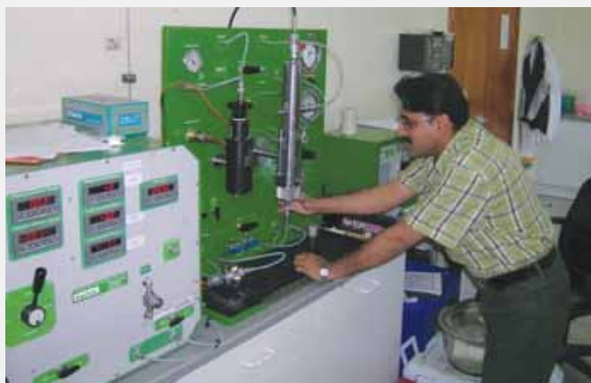
Senior Core Analyst Ismail Azam is measuring rock permeability at ResLab's laboratory in Abu Dhabi.
