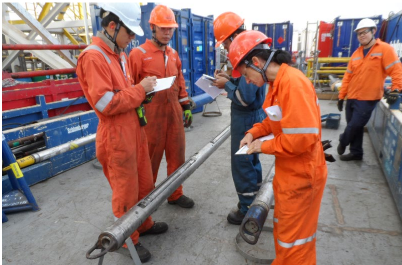
Retrieving reservoir fluid samples from the wireline tools is a critical part of the formation evaluation process.
