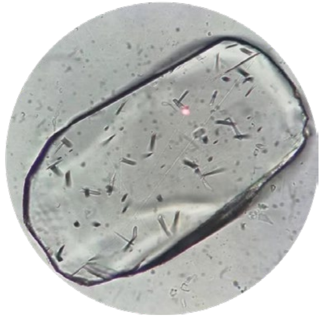
Apatite crystal showing evidence of uranium decay. The short, dark linear features are fission tracks. Fission tracks are formed when an uranium atom splits into two large nuclei. Helium is not released during this process. However, the number of fission tracks is an approximate for the total uranium content of the mineral. It is known that only roughly one in two million uranium atoms decay through spontaneous fission. This indicates how much uranium is present in the mineral and as a consequence how much helium has been formed. The crystal is ~150µm in length.
