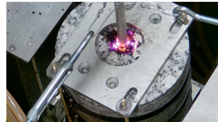
Laboratory test facility where the millimetre wave drilling technology is being tested.
