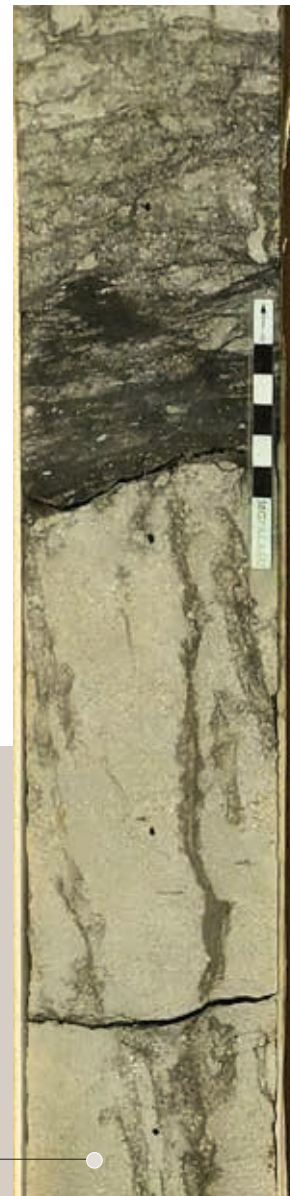
Contact between the Kingia Fm and the overlying Irwin River Coal Measures, marked by an extensive network of Ophiomorpha . Well Waitsia 3, 3239 m.
