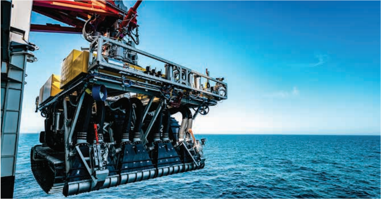
This collector was a key piece of the pilot nodule collection system trial carried out by The Metals Company and Allseas in the CCZ in September last year.
