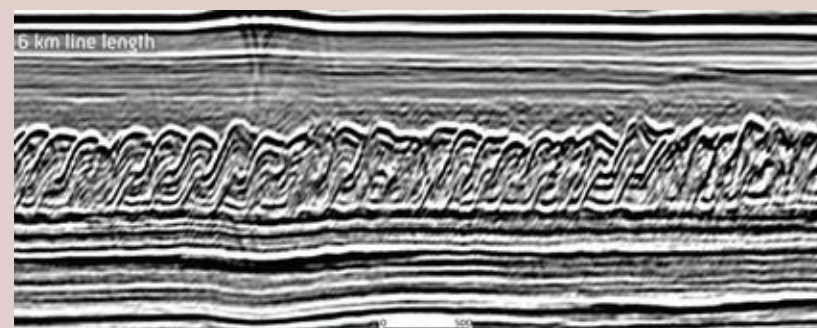
Figure 3: Searcher 2023 reprocessed seismic line with a recent MTC in the Krishna Godavari Basin of East India. Appearing structure and characterless when viewed in its entirety (ca 200km long), in detail at near 1:1 ratio individual thrusts with a thrust angle near 45° can be observed. Note the erosive base of the MTC cutting into and truncating the sand rich basin floor meandering channel systems running almost coast parallel in this basin.
