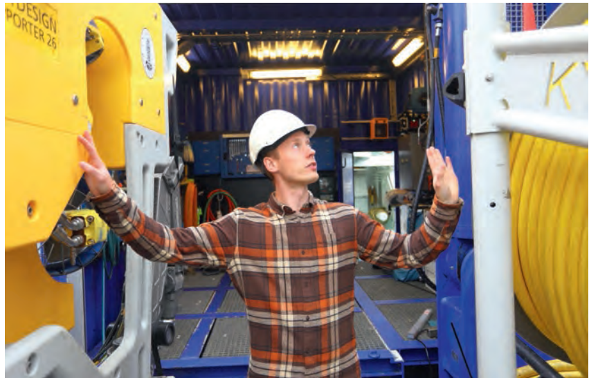
PhD scholar Håvard Hallås Stubseid inspects the university's ROV (left), which can dive to a depth of 6,000 metres. On the right is the tethering equipment known as the Tether Management System, to which the ROV is connected when it carries out subsea operations.
