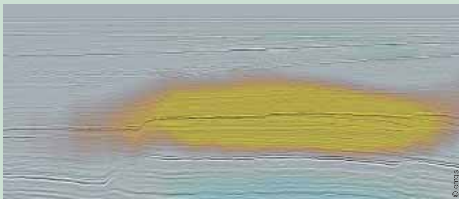
Depth migrated image from a one line survey across the giant Troll field in the North Sea. The reservoir is in Upper Jurassic sandstones situated below the prominent reflector in the middle of the section. The hydrocarbon filled reservoir at a depth of approximately 1000m has resistivities approaching 250 \Omega m, while water wet sandstones and overburden shales have resistivities in the order of 1-2.5 \Omega m.
