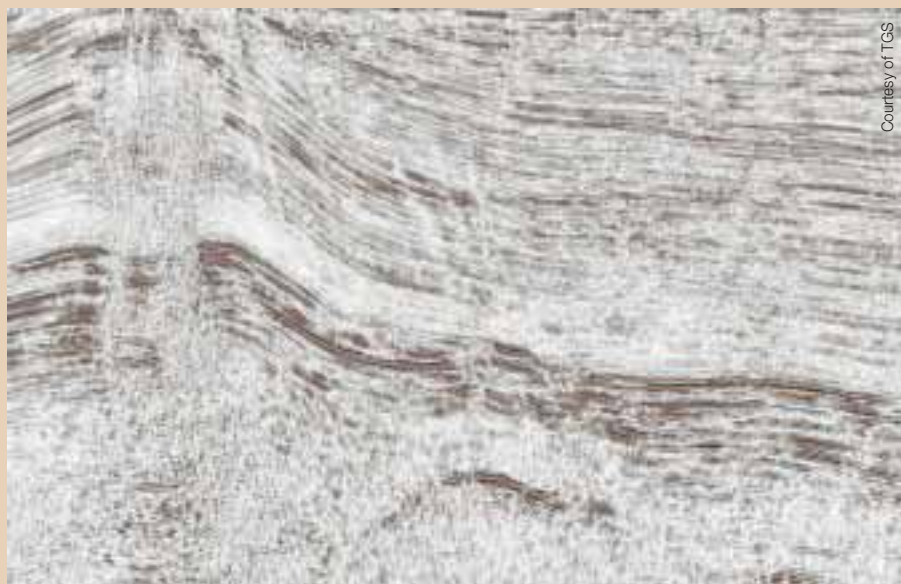
Seismic line through the Lunskeye gas-condensate field offshore Sakhalin shows the gas cloud above the proven field and channel deposits immediately to the east, not imaged on older vintage seismic in the area.
