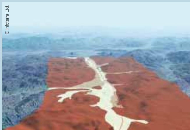
3D visualisation using satellite imagery is very valuable when undertaking landcover and elevation analysis for pipeline route planning.
