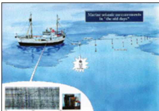
Acquisition technology as used in a 1969 Svalbard survey. Illustration by Anders Farestveit.
