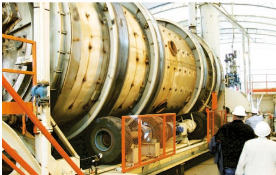
The ATP processor similar to what will be used to retort oil shale in Utah.
