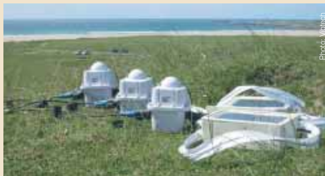
Photo: Vibtech Cellular SeismicTM - Vibtech testing and performing production trials with Unite, their cable free seismic system, using mobile networking technology.
