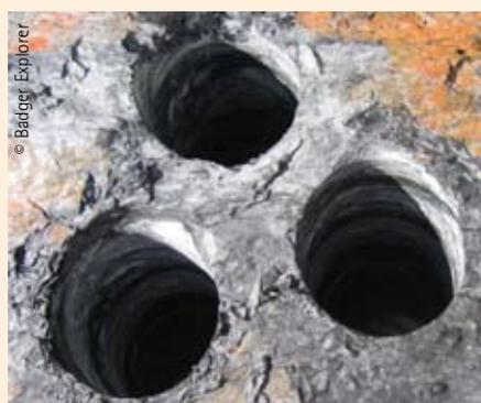
Test holes made by Badger Explorer. There is no need for drilling mud or casing.
