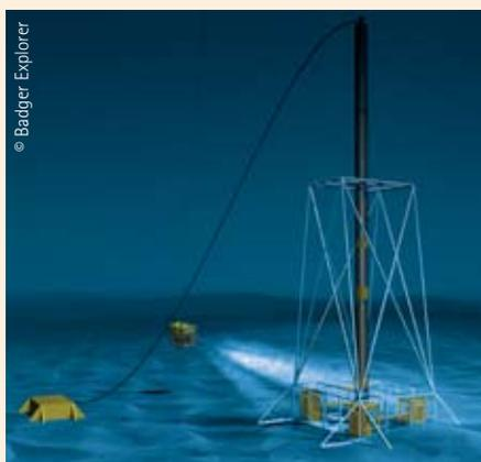
Badger Explorer, about 30m long with a diameter of 15cm, is transported to the drilling location by boat and then lowered on wire to the sea floor and put in a start position assisted by ROV and a guide frame.
