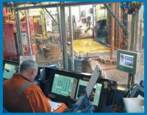
The drilling of wells from Gullfaks A is utilizing modern technology that is highly automatic involving a minimum of personnel. All drilling parameters are shown on monitors watched by the drilling supervisor and his crew.
