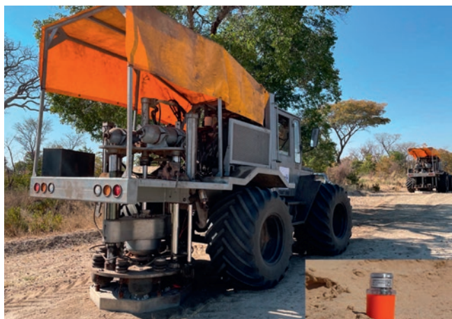
Accelerated weight-drop seismic source – the Polaris Explorer 860. This source is highly manoeuvrable and requires only 3 metres wide access tracks. The receivers being used are wireless Stryde Nodes (insert image), which are small and compact even by the standards of modern nodes.
