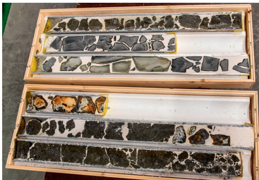
Resinated cores collected from the NPDs drilling campaign at the Mohns Ridge in 2020. Darker areas are sulphide materials, while the lighter grey are basaltic rocks.
