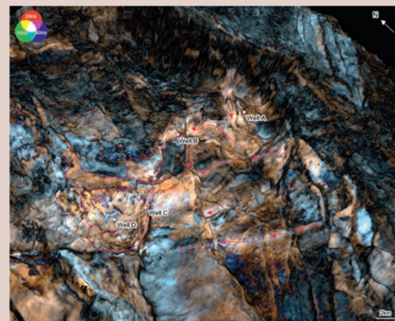
Figure 1. Spectral decomposition RGB-blend on an Upper Jurassic surface. Sediment-routing systems are shown by the magenta dashed arrows and submarine lobe systems are shown within dashed magenta lines.
