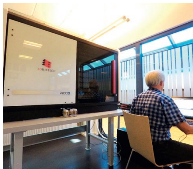
The author at the controls of the Norwegian Petroleum Directorate's 3DHistech P1000. This scanner has a capacity of 1000 standard microscope slides, and scans at 0.25 µm per pixel at a numerical aperture of 0.95. Scan time for each focal layer of 330 square millimetres is two minutes.
