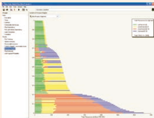
Example from GeoX - Visualization of results from assessment of a prospect with 4 segments, showing the contribution of resources from each segment and the distribution and total resources.
