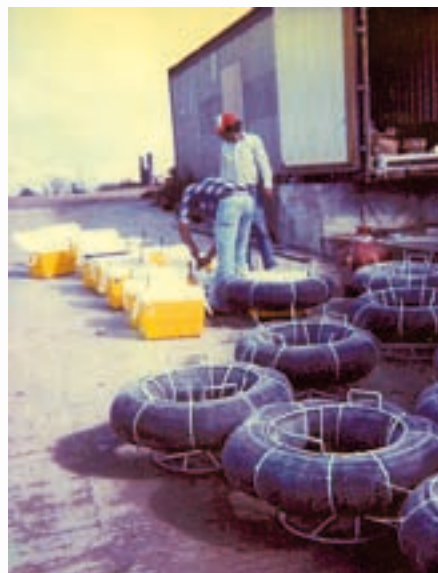
Offshore deployment of seismic group recorders with floatation collars.
