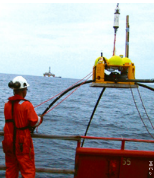
Multi component receiver is seen being deployed from the survey vessel.
