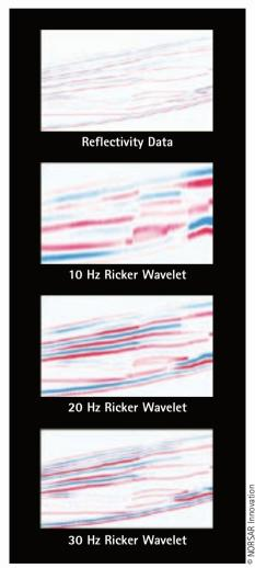
For a given target model and illumination coverage, SimPLI generates a set of images for a range of pulses. High pulse frequency results in better resolution, but the software makes it possible to quantifiably determine the effect of the pulse frequency on the 3D PSDM image (data courtesy of the SVALEX project, sponsored by Statoil).
