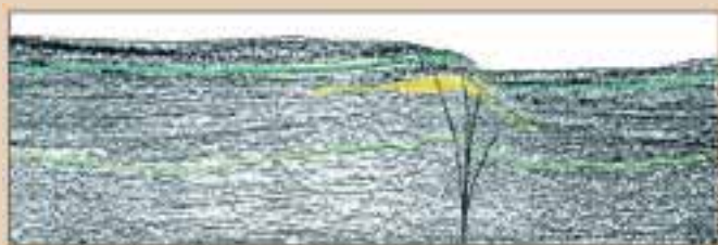
Wrench Fault anticline in deep water.
