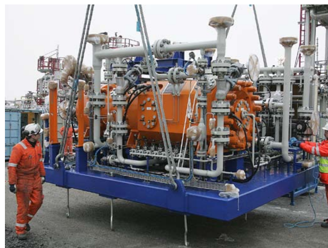
Installation of subsea compressor at the K-lab testing facility, prior to contract award.
