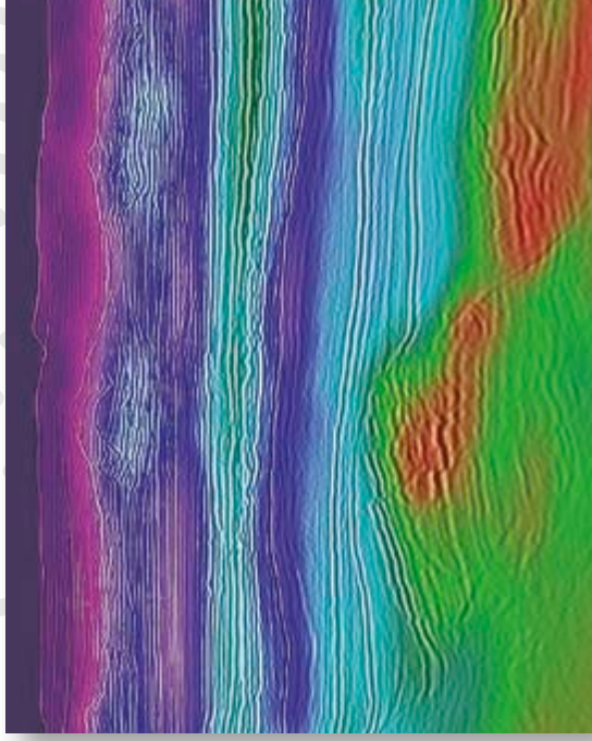
Application of GX Technology's high resolution tomography using accurate general move out picks resolves small-scale velocity heterogeneities.
