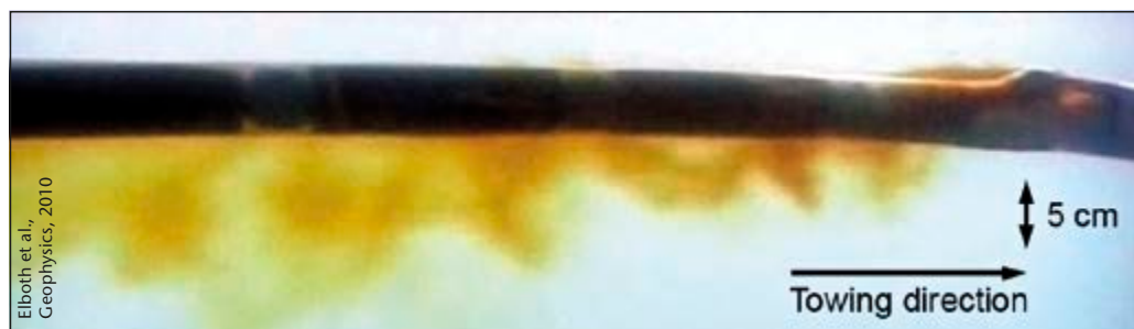
Figure 3: Turbulent flow around a seismic streamer, visualised by a single hole dye release.
