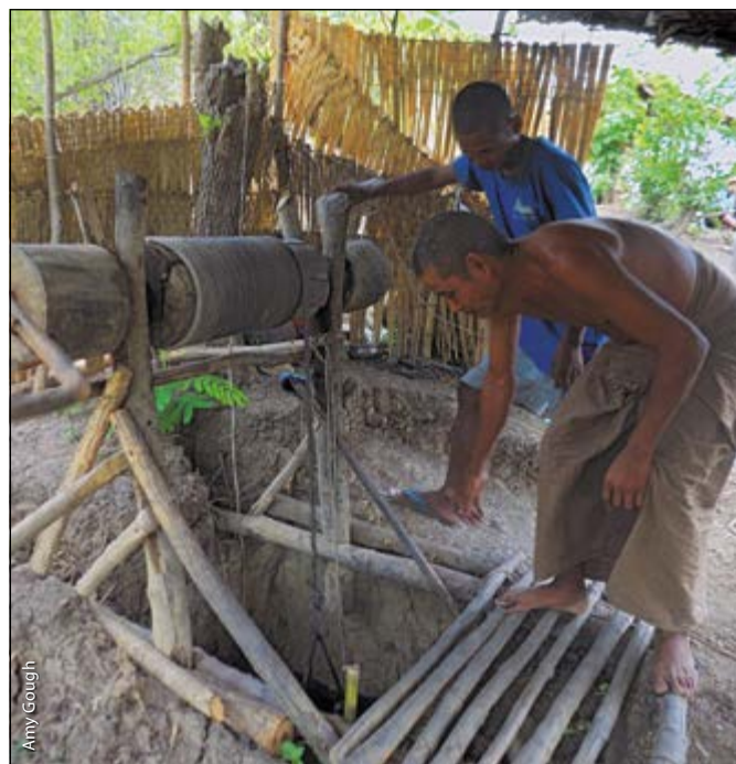
A Yenangyuang oil well dug by hand using metal-tipped bamboo rods attached to a small generator.
