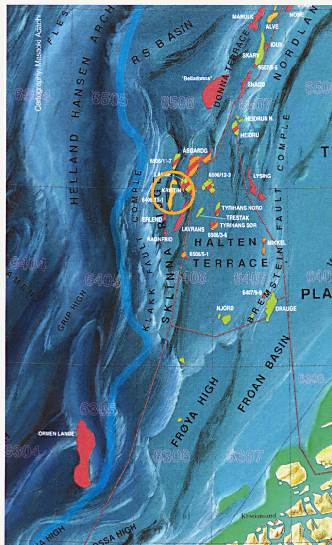
Structural map of the Norwegian Sea shows the relief at the base Cretaceous level. The 500 m contour drawn on top of the geological features separates shallow water from deep water (blue curve). The Norwegian independent Saga Petroleum discovered Kristin in 1996. It is located next to a number of other Norwegian Sea oil and gas fields within the geological province named Halten Terrace.
